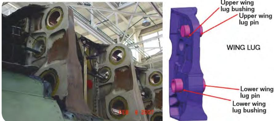
FIGURE 1 Corrosion in F-18 wing-fuselage attach bulkheads.<sup>8</sup>
