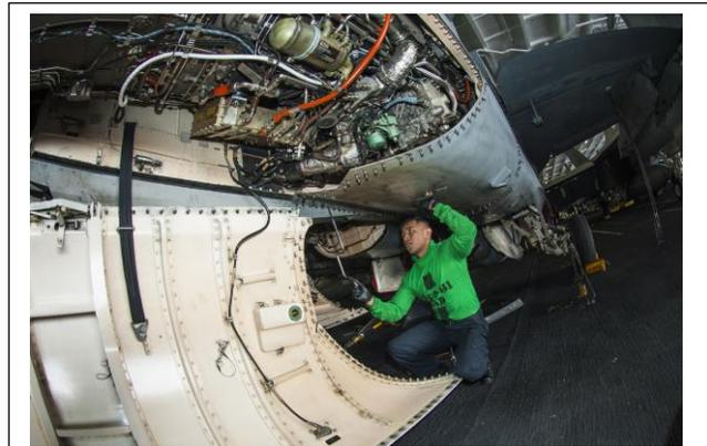
Figure 2 84-day corrosion inspection on an F/A-18E Super
