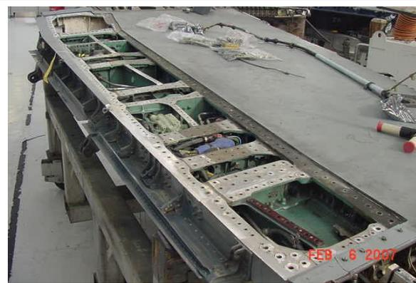
Figure 3 Corrosion under F/A-18F wing panels
