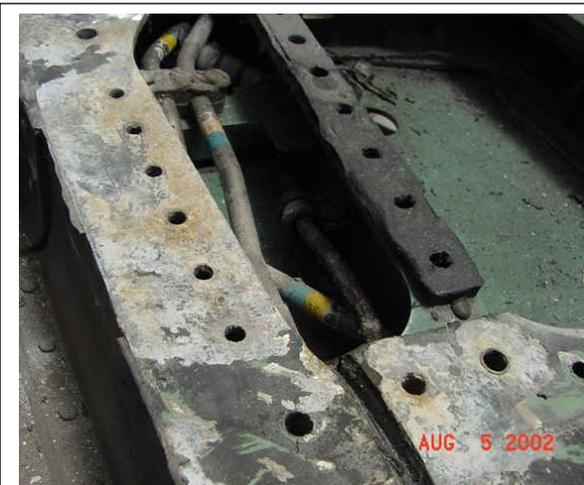
Figure 4 Close-up of corrosion under F/A-18F wing panels
