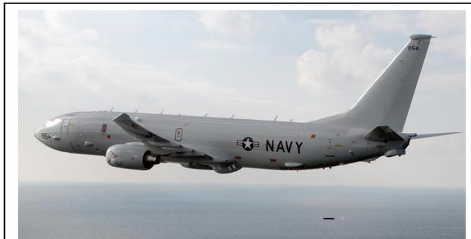
*Figure 1 P-8 launches a sonobuoy over the Atlantic Test Range*
