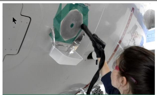
Figure 2 Selective non-drip anodizing applied directly on plane
